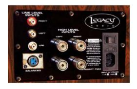
NOTE: When using the LFE input, the freq. control on the front panel of the Xtreme XD will be bypassed. The level control will then function as a sensitivity control, allowing the preamp/processor to control volume.
